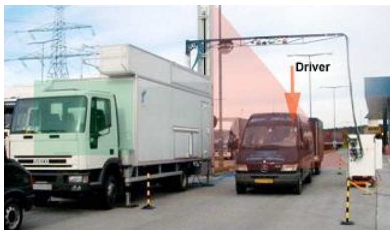
Picture 2 – Silhouette scanner type – (300 keV) transmission dual energy x-ray unit, continuous exposure. The driver sits inside the scanned vehicle while driving it through the scanner.
