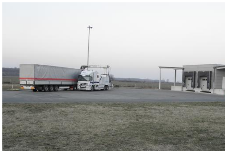
Picture 4 – LINAC, high-energy x-ray scanning unit type – 4.5 MeV pulsed exposure. Driver is not inside the stationary cargo truck.
