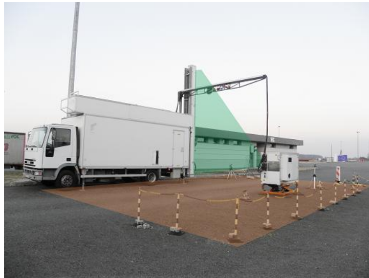
Picture 3 – Silhouette scanner type – 300 keV transmission x-ray unit, continuous exposure. Exclusion zone around the full operational unit is shown.
